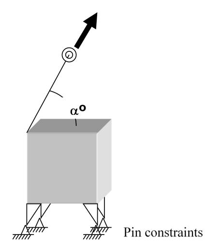
Figure 3: Load Case #2 – Gondola Single Cable Loading
