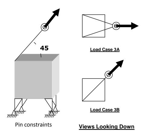
Figure 4: Load Case #3 – Off-Vertical Gondola Loading
