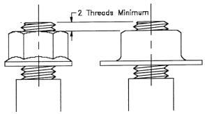
Figure 2.3-1 Minimum Bolt Thread Protrusion through Self-Locking Nuts and Nut-Plates
