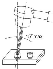
Figure 1.3-2 Torque wrench angle
