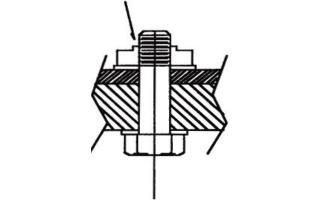
Figure 2.3-2 Grip Length Requirements for Bolts in Bearing
