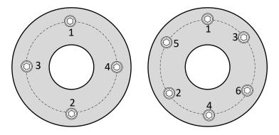
Figure 2.5-1 Tightening Sequence
